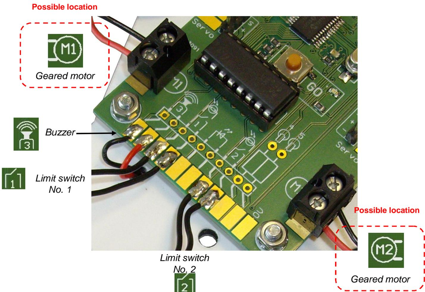
**Connecting the line tracer, buzzer and geared motor:**
