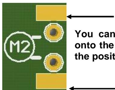
You can solder the geared motor wires directly onto the rectangular pads shown on either side of the position for the 2-pin terminal.
