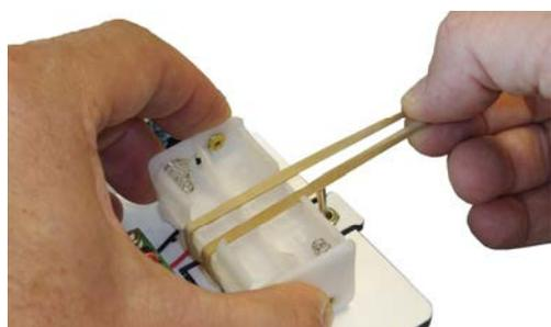
Pull the elastic band and pass it under the switch.
