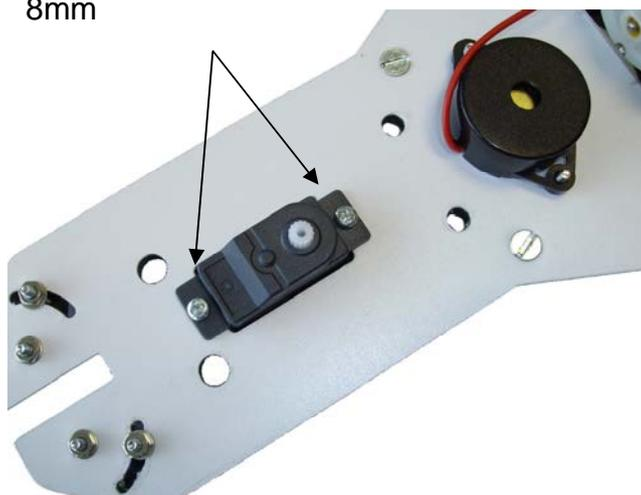
The spindle of the servomotor should be facing the buzzer.
