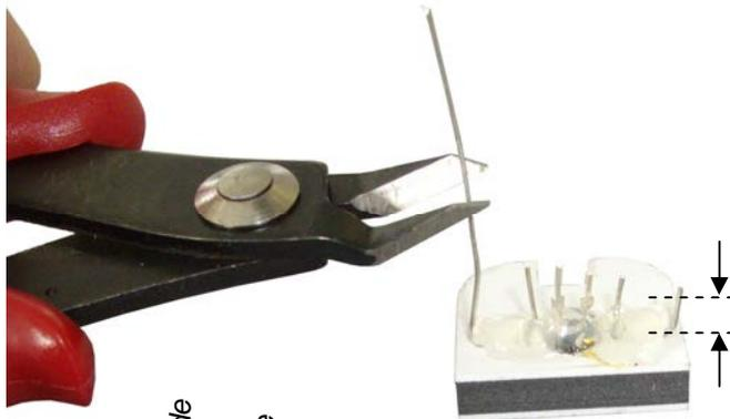
Trim the pins of the components 5mm above the level of the hot glue.
