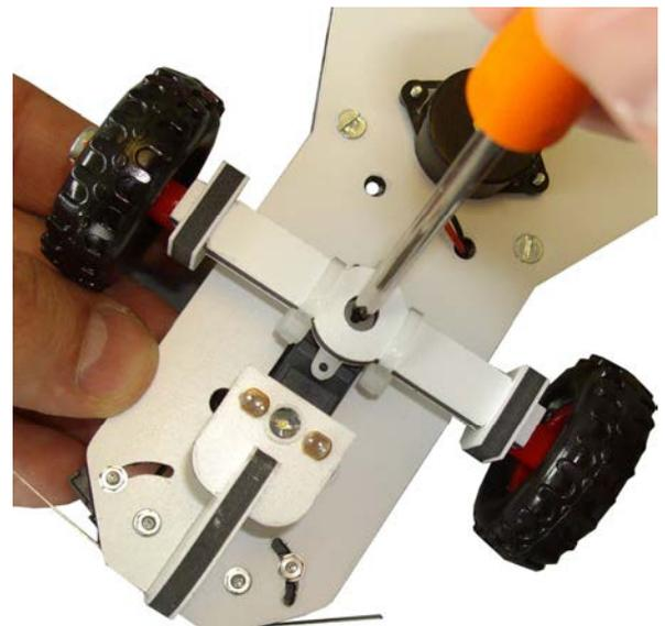
Tighten the screw which was supplied with the servomotor through the axle
