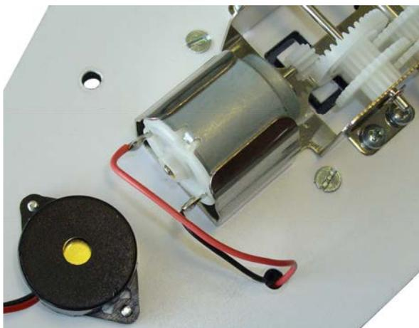
Thread the wires through one of the two holes located on each side of the geared motor.
