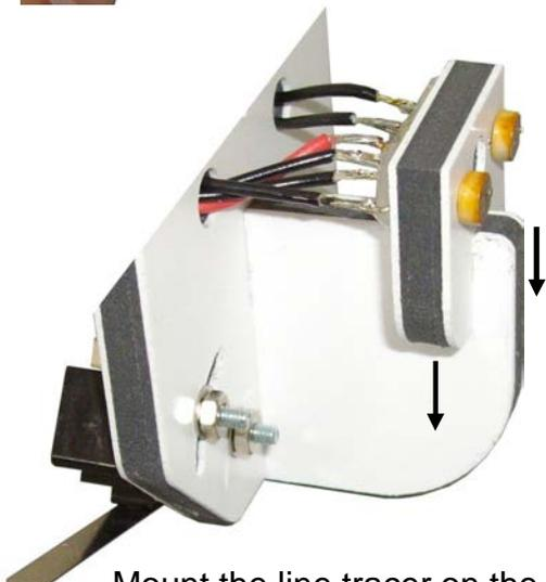
Mount the line tracer on the nosepiece.
