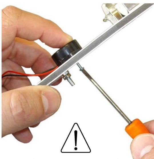
Depending on our supplies, the fastening lugs on the buzzer may have a larger diameter than the screws. In this case, put an M2 nut on the end of each screw.
