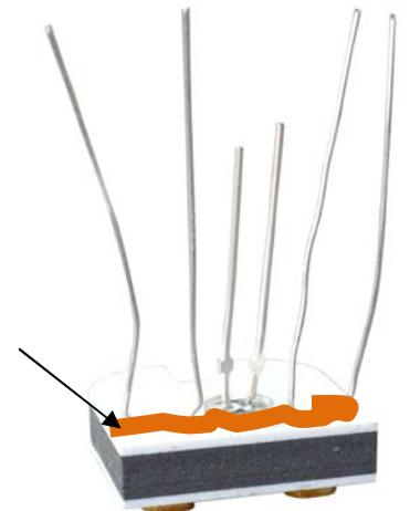
**Before gluing, identify the anode and cathode of the white LED.**
