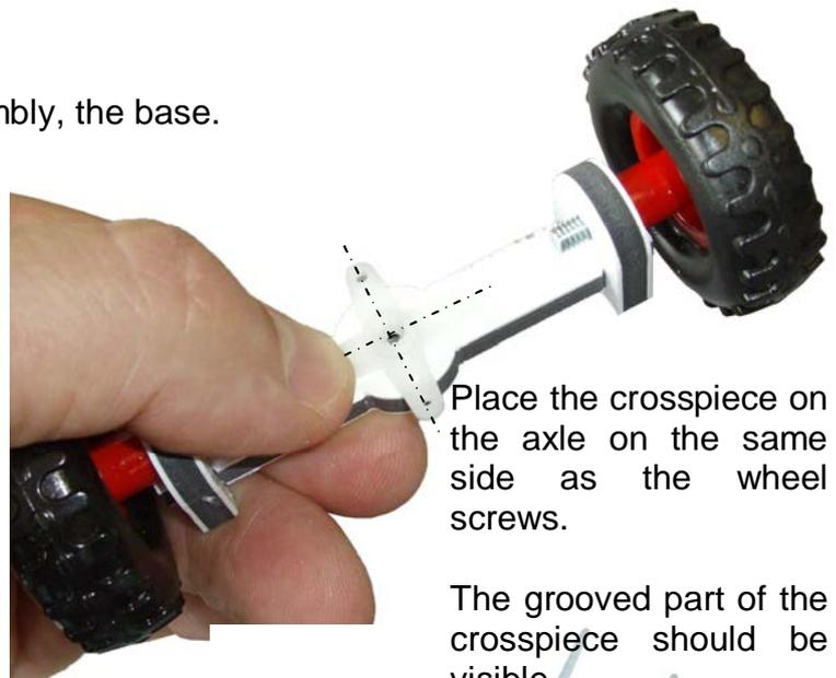
From the mechanical parts supplied, take the crosspiece and the fastening screw
