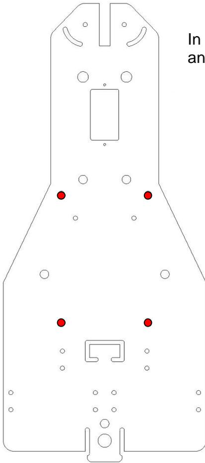
In the places marked below, screw one M3 x 14mm countersunk screw and 2 M3 nuts per position into the base (A).
