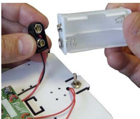
Connect the 9V clip to the battery holder.
