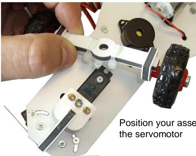
Position your assembly on the servomotor
