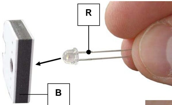
On the line tracer mounting (B), insert the white LED (R) into the largest hole.
