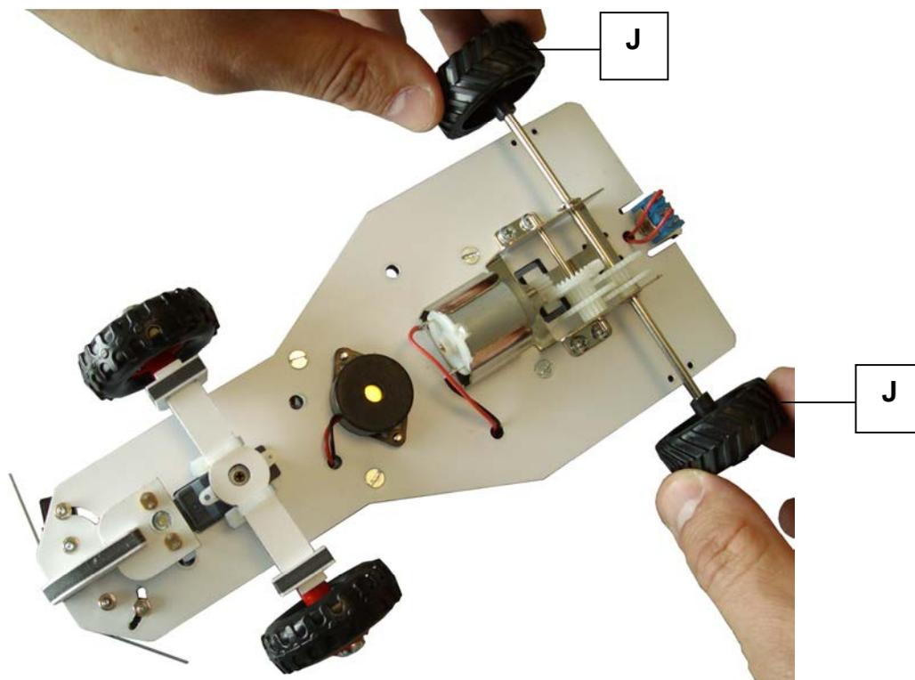
Push the wheels (J) onto the geared motor's axle.
