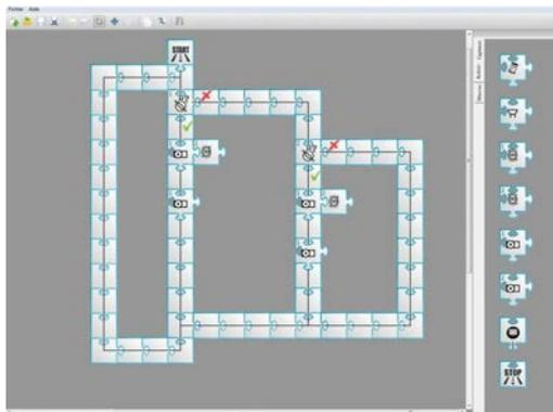
Connect your PC using a USB 2.0 AB cable, ref. 283476, the intuitive visual programming software will allow you to easily program your circuit board based on your wiring.
