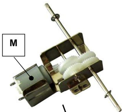
Mount the geared motor (M) in the position marked on the base
