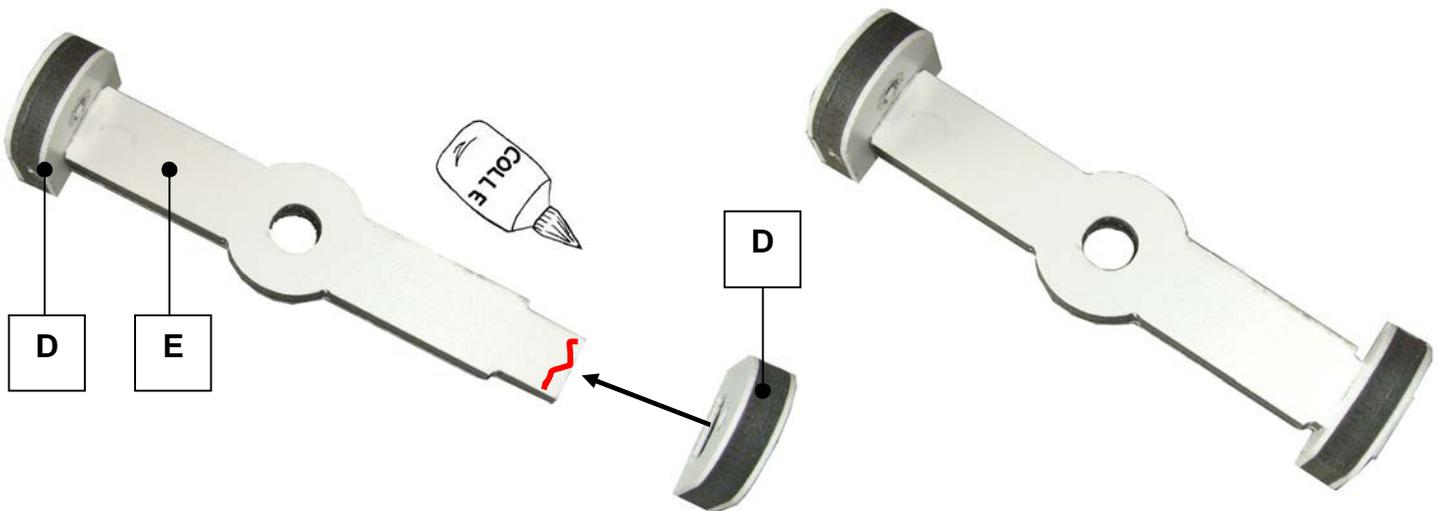
Push the wheel mountings (D) onto each end of the front axle (E): the holes on the wheel mountings should be facing the same side.
