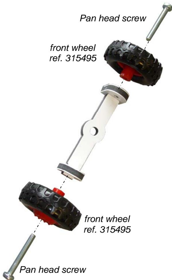
Using the 2 pan head screws M4 x 30mm, attach the wheels to each wheel mounting: by fully tightening the two screws, they tap into the mountings (D).
