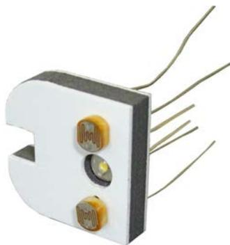
The two LDRs should be stuck onto the mounting.
