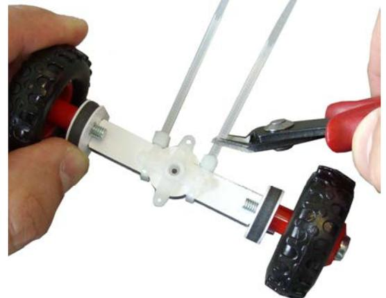
Do the same for the second branch and then cut off the excess cable tie using cutting pliers.
