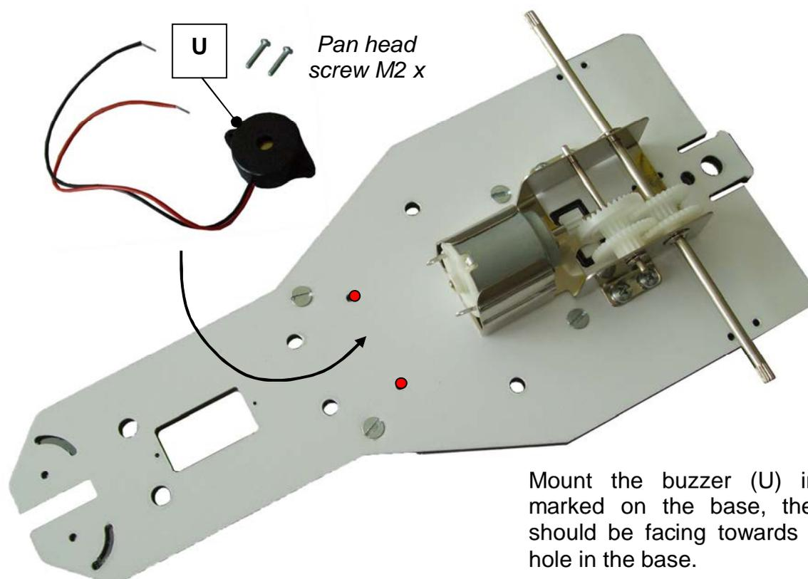
Mount the buzzer (U) in the position marked on the base, the buzzer wires should be facing towards the rectangular hole in the base.
