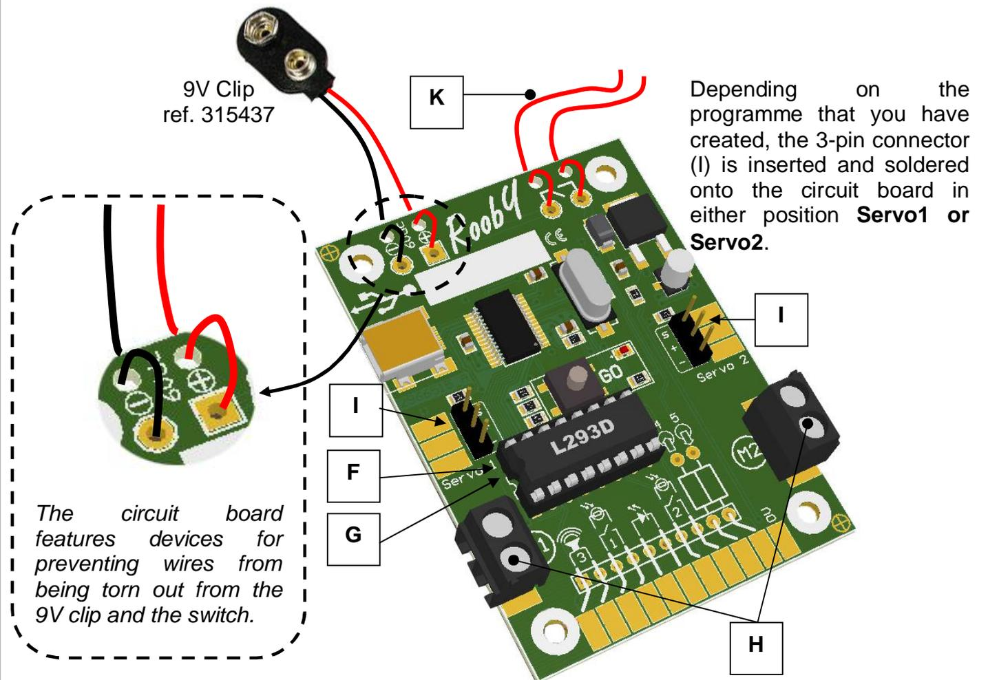
Depending on the programme that you have created, the screw terminal (H) is inserted and soldered onto the circuit board in either position **M1** or **M2**.
