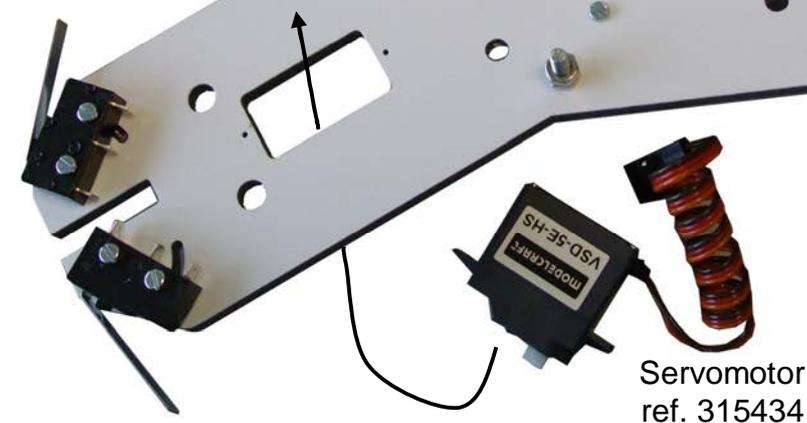
The servomotor is inserted into its position on the base.
