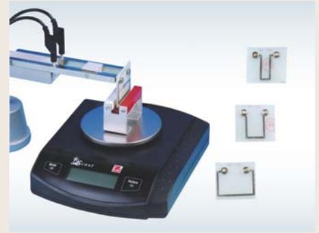
With 4 interchangeable printed conductors (1, 2, 4 and 8 cm). The holder is turnable in a horizontal and vertical position. Complete with a set of 6 removable permanent magnets in holder. The maximum current is 5A.
